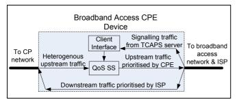
Figure 3: CPE block diagram
