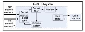
Figure 4: Simplified QoS SS block diagram
